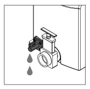
front of the machine to drain any excess water from the pump. •
