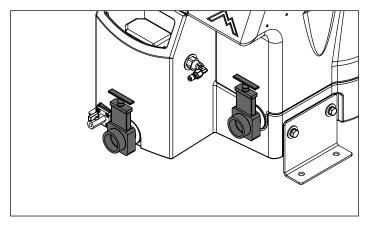
The Escape® Plus features tank drain valves on the recovery and solution tanks. The pump-out can also be used to empty the recovery tank. ◆
