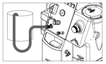
Connect a garden hose to the pump-out fitting on the front of the machine. The other end of the hose can be placed in a holding tank for recovered water. Switch on the **PUMP-OUT** and open the ball valve. Recovered water
