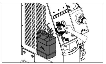
Fill the included 7 qt. bottle with chemical concentrate of your choice. With a cleaning tool connected, switch on the pump and pull the trigger on your tool to keep water flowing. Turn the chemical injection knob counter-clockwise to open the valve. This allows chemical to siphon into the line. Turn the knob until you see the bubble reach the desired gallons per hour of chemical. Follow chemical manufacturer's instructions for correct ratio.
