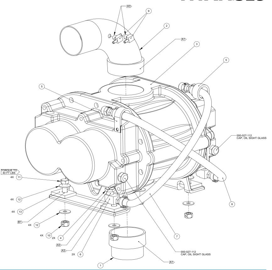
**Figure 8-12. Blower Assembly - View 2 of 2** 610-002-725 Rev. G -BLOWER (0.333) -<u>B1</u>>2X TORQUE TO 30 FT LBS (0.573) -COUPLER END OF BLOWER SHAFT FLUSH WITH INSIDE OF COUPLER - B1> 3X -B1>2X TORQUE TO 30 FT LBS (0.925) ENGINE-
