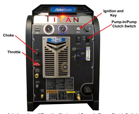
Figure 3-1. Location of Throttle, Choke and Pump-In/Pump Clutch Switch
