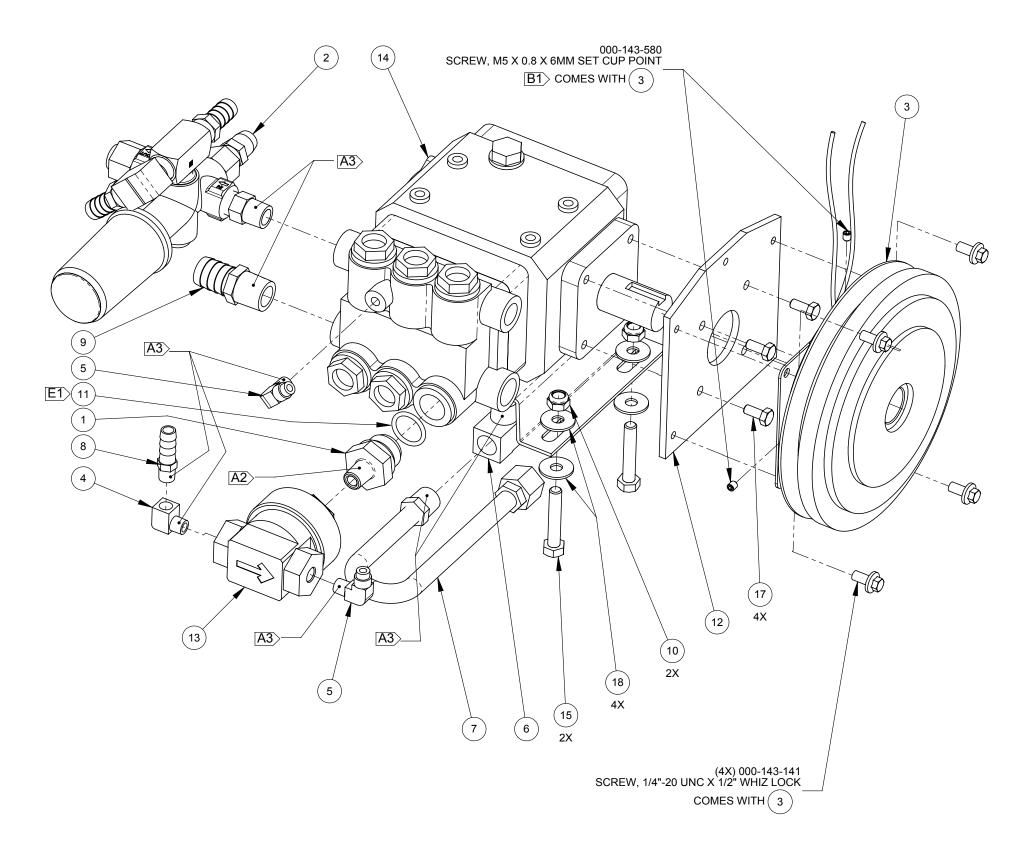
**Figure 8-9. Pump Assembly - View 2 of 2** 610-007-737 Rev. B
