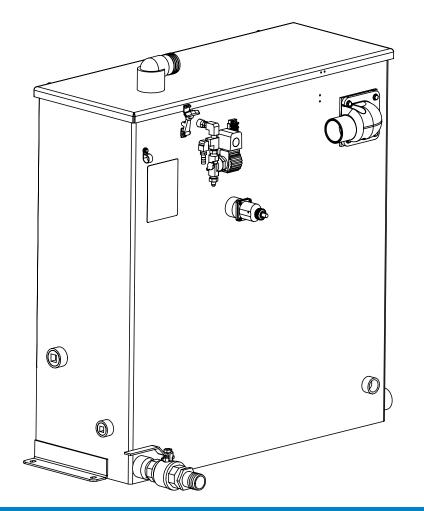
Figure 8-28. 70 Gallon Universal Recovery Tank (URT) Cover Assembly 610-029-726 Rev. B
