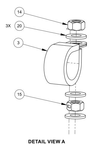
TITAN.325 000-049-053 FILTER, B&S VANGUARD FOAM AIR FILTER-000-049-014 FILTER, OIL B&S-2X (20) 17 TORQUE TO 25FT LBS
