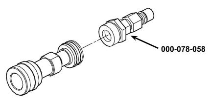
Figure 4-2. Recirculation Fitting
