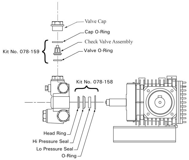
Figure 4-1. Servicing the Valves
