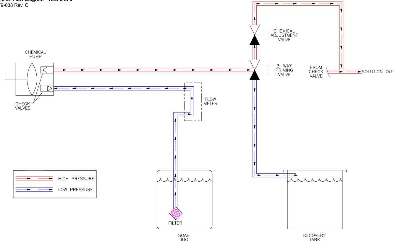
Figure 5-3. Flow Diagram - View 3 of 3 000-179-038 Rev. C
