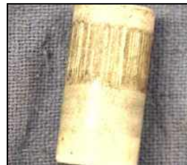
Figure 5-8. Examine Ceramic Plungers
