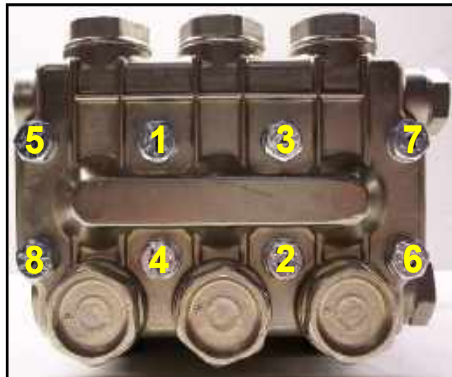
Figure 5-17. Torque Sequence in "X" Pattern
