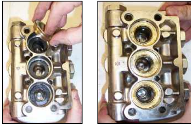
Figure 5-14. Install Retainers into Cavities
