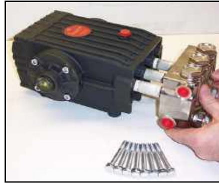
Figure 5-16. Re-install Manifold and Torque Fasteners
