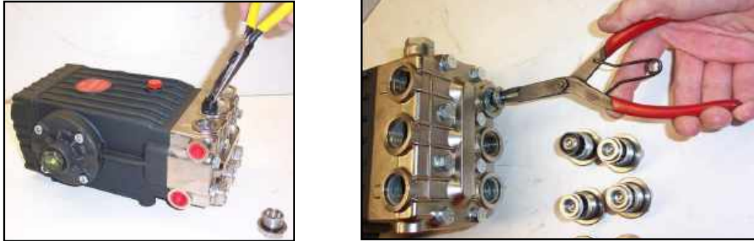
Figure 5-1. Remove Valve Cap and Valve Assembly
