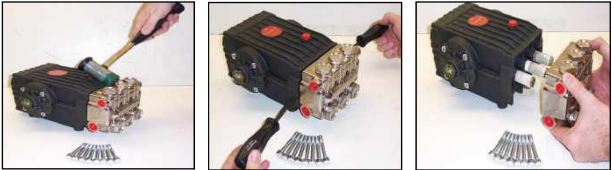
Figure 5-6. Separate Manifold from Crankcase
