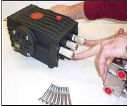
Figure 5-16. Re-install Manifold and Torque Fasteners
