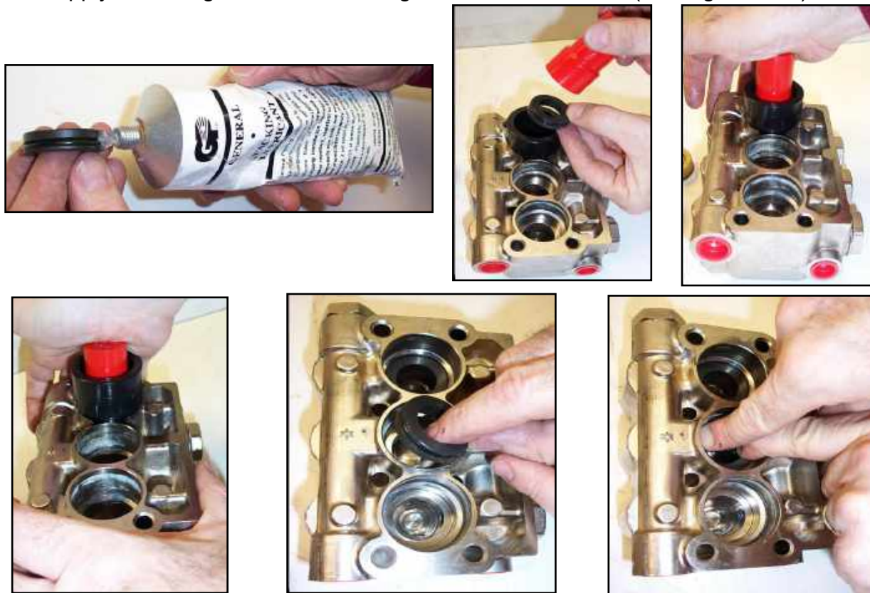
Figure 5-13. Install Seal Assembly Using O-Ring Grease
