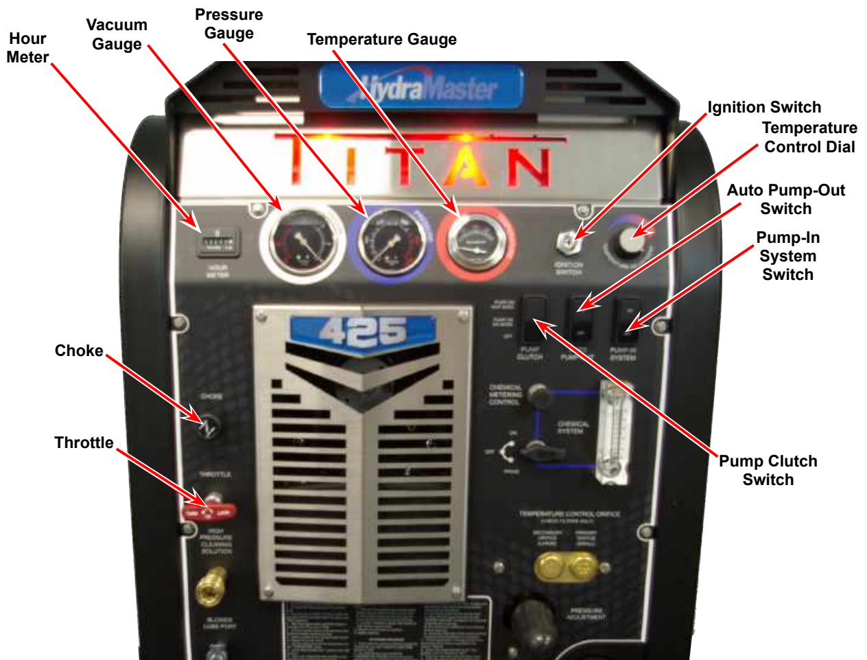
Figure 4-1. Titan 425 Upper Dash Assembly
