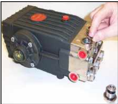
Figure 5-4. Apply Grease and Install Valves
