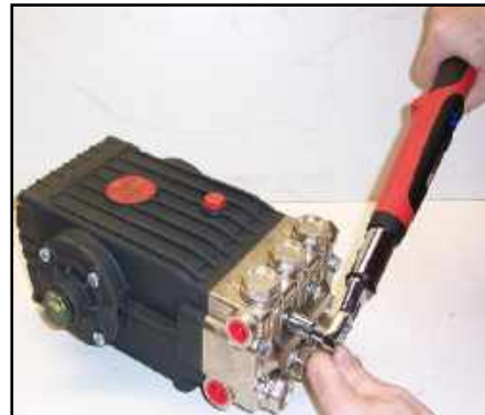
Figure 5-18. Torque Bolts to 22 ft. lbs
