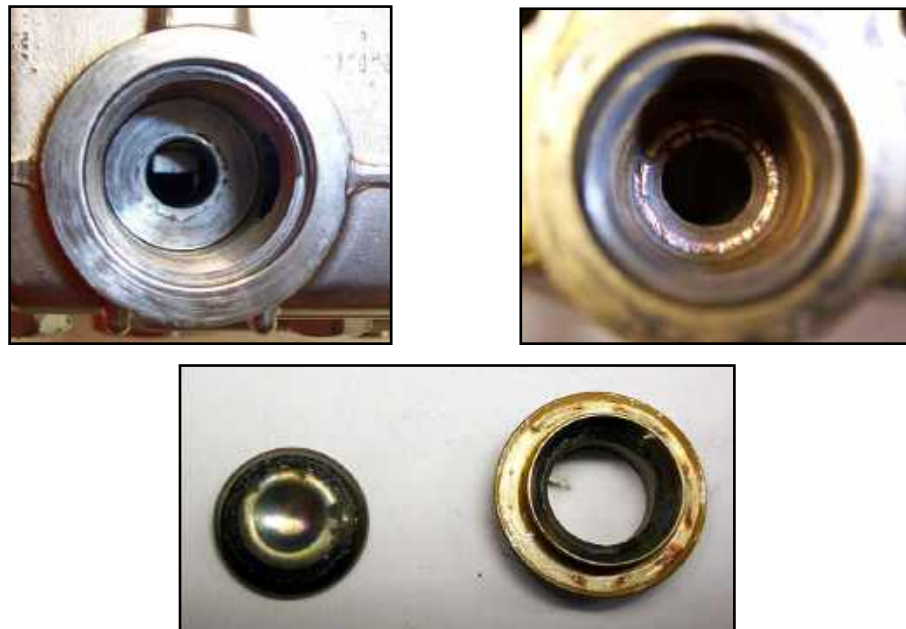
Figure 5-2. Inspect Manifold and Old Valves
