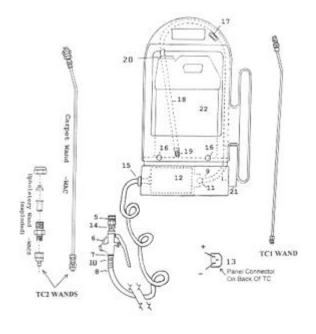
ALWAYS PLUG IN THE TC BETWEEN JOBS. THE #B924 GEL CELL LEAD ACID BATTERY ALWAYS WANTS TO HAVE A FULL CHARGE. LEAVING THE #B924 HUNGRY SHORTENS ITS LIFE. IT IS IMPOSSIBLE TO OVERCHARGE THE #B924. DO YOU WANT THE OPTION TO CHARGE THE TC IN THE SHOP? RADIO SHACK SELLS A BASEBALL SIZED AC TO DC CONVERTER WITH A CIGARETTE LIGHTER ORIFICE FOR ABOUT \$30. PART # 22-165.
